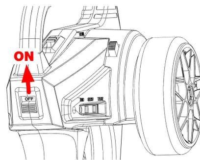
1. CONNECTEZ LA BATTERIE AU CONTRÔLEUR
